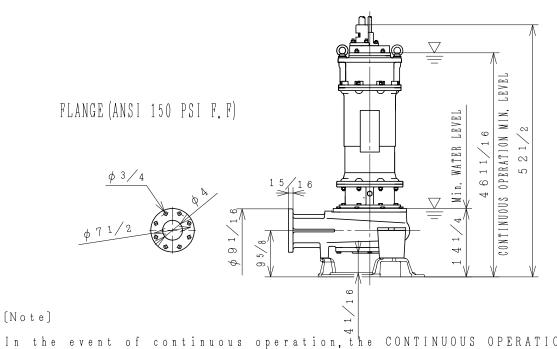
In the event of continuous operation, the CONTINUOUS OPERATION MIN. LEVEL must be maintained.
