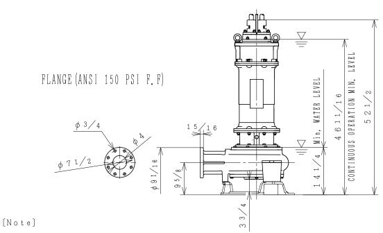
In the event of continuous operation, the CONTINUOUS OPERATION MIN. LEVEL must be maintained.
