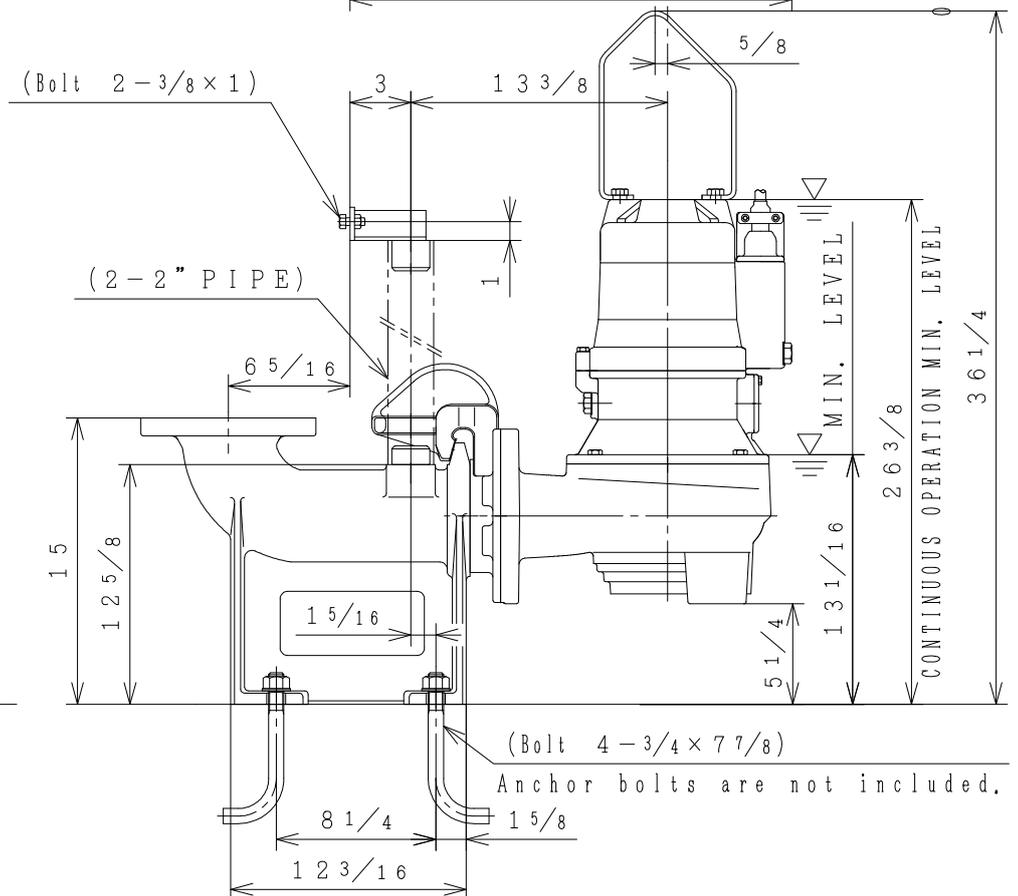
[Note] Limit operation to 30 minutes (maximum) when operating the pump between the MIN. LEVEL and CONTINUOUS OPERATION MIN. LEVEL. In the event of continuous operation, the CONTINUOUS OPERATION MIN. LEVEL must be maintained. Cables are not shown on this drawing.
