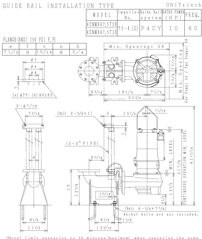
[Note] Limit operation to 30 minutes (maximum) when operating the pump between the MIN. LEVEL and CONTINUOUS OPERATION MIN. LEVEL. In the event of continuous operation, the CONTINUOUS OPERATION MIN. LEVEL must be maintained. Cables are not shown on this drawing.
