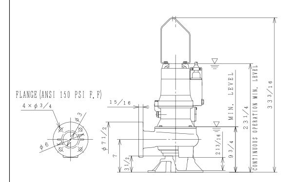
[Note] Limit operation to 30 minutes (maximum) when operating the pump between the MIN. LEVEL and CONTINUOUS OPERATION MIN. LEVEL. In the event of continuous operation, the CONTINUOUS OPERATION MIN. LEVEL must be maintained. Cables are not shown on this drawing.
