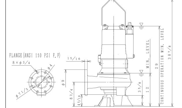
[Note] Limit operation to 30 minutes (maximum) when operating the pump between the MIN. LEVEL and CONTINUOUS OPERATION MIN. LEVEL. In the event of continuous operation, the CONTINUOUS OPERATION MIN. LEVEL must be maintained. Cables are not shown on this drawing.
