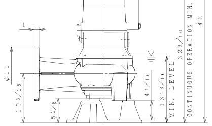
[Note] Limit operation to 30 minutes (maximum) when operating the pump between the MIN. LEVEL and CONTINUOUS OPERATION MIN. LEVEL.
